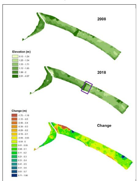
Figure 4. Elevation and change in elevation of the San Pablo Bay shoreline, 2008-2018. The grain/grid cell size is 5 m x 5 m. The purple box over a portion of the 2018 elevation map represents the area flown using the UAV. miles of SR 37 lost elevation (0.1 to 1.8 m) between 2008-2018.
