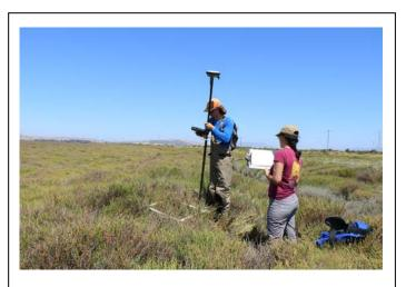
Figure 1. Using the RTK-GPS in a tidal marsh on the San Pablo Bay shoreline.
