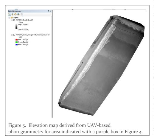
elevation map was much higher resolution than the equivalent elevation map derived from field RTK-GPS measurements. Both are much higher horizontal and vertical resolution than typical elevation maps from airplane-based LiDAR (typically 1 meter<sup>2</sup> horizontal and 10 cm vertical, RMSE).
