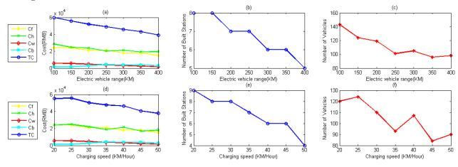
Figure 9 Sensitivity of cost components to parameters C (sub-figures (a)-(c)) and F(t) (sub-figures (d)-(f))
