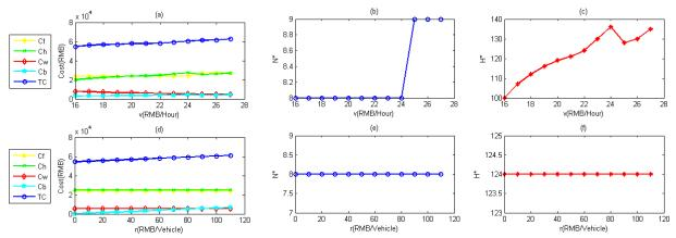
Figure 8 Sensitivity of cost components to parameters  $\mathcal{V}$  (sub-figures (a)-(c)) and r(sub-figures (d)-(f))
