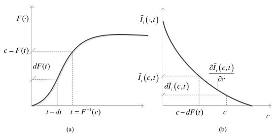
Figure 1. Illustration of how EV charging affects the change of  $\tilde{I}_i(c,t)$  over time.
