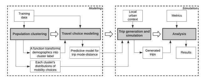
Figure 1. Data-driven modeling and simulation framework.
